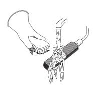
The cable and outer surfaces of the AV Sensor may also be cleaned with mild detergent and warm water.
